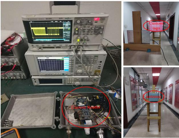
Fig. 7. RFID hardware setup used in the experiments
