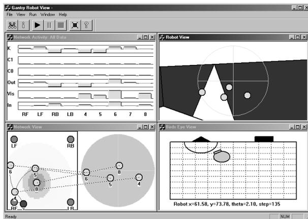
**Figure 1** Screen shot of the simulated arena and robot. The bottom-right view shows the robot position in the arena with the triangle and square. Fitness is evaluated on how close the robot approaches the triangle. The top-right view shows what the robot “sees,” along with the pixel positions selected by evolution for visual input. The top-left view shows the instantaneous activity of all nodes in the neural network. The bottom-left view shows the robot control neural network.
