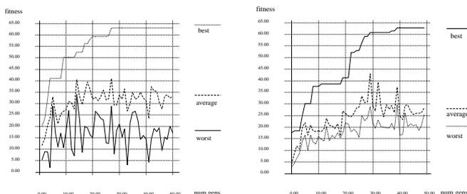
Figure 7: Comparative results for different fitness functions. Left-hand graph is where fitness is measured by the *average* of a series of tests; right-hand graph where fitness is measured as the *worst* performance in a series of tests. Abscissa is generation number; ordinate is fitness value. See text for further explanation.
