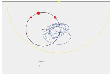
**Fig. 6.** Line patterns generated by a robot that had to perform obstacle avoidance and phototaxis in order to find the target regions where its lines would gain the maximum fitness. The top of the image is the arena wall, the dot on this wall represents the light and the semicircular area is the target region. Note that the robot marks a small curved line on the way to the light. The robot is the circle with the dot at its centre.
