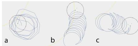
**Fig. 2.** Line patterns generated in simulation using an ecological fitness function and a simple motor model. a) is the typical pattern generated by a 20 neuron network; b) is an ‘orange segment’ pattern occasionally (approximately 30%) generated by a 20 neuron network; c) is the typical pattern generated by a 40 neuron network (which after further evolution looks like Figure 3). The robot is the circle with the dot at its centre.
