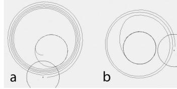
**Fig. 5.** Line patterns generated in simulation with a 20 neuron network and a more sophisticated motor model with inertia and momentum. The robot is the circle with the dot at its centre.
