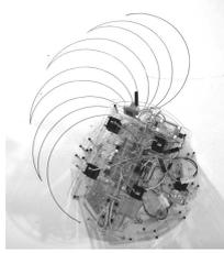
**Fig. 3.** Top-down view of an ‘orange segment’ line pattern generated by a Drawbot in the real world which was evolved in simulation using the implicit ecological fitness function, a 40 neuron network and a simple motor model.
