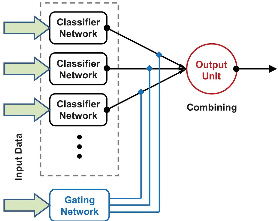
**Fig 1. The standard MoE architecture.** The outputs (classifications) from the classifier networks are fed into an output unit which combines them according to some simple rule. The gating network weights the individual classifier outputs before they enter the final output unit, and thus guides learning of the overall combined classification. The classifiers and gating networks receive the same input data. See text for further details.
