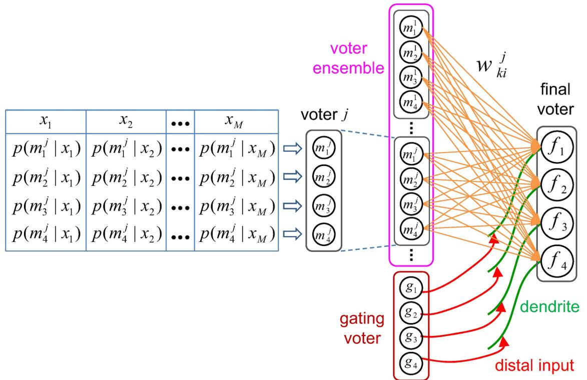
**Fig 3. A voter and the voter ensemble network ( $N_C = 4$ ).** (Left) A voter and the predefined firing probabilities of each voter neuron for a set of virtual input samples  $X = \{x_1, x_2, \dots, x_M\}$ . (Right) The voter ensemble network. The weight  $w_{ki}^j$  represents the weight of connection from the  $i$ th neuron of the  $j$ th voter to the  $k$ th neuron of the final voter.
