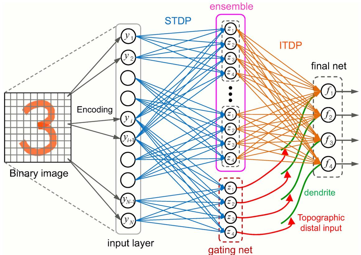
**Fig 4. SEM-ITDP ensemble network architecture.** The STDP connections, which projects from the selected input neurons to each WTA circuit, together with the WTA circuits constitute the SEM ensemble. The ITDP connections have the same connectivity as the logical ITDP model. All of the ensemble, gating and final output networks use the same SEM circuit model.
