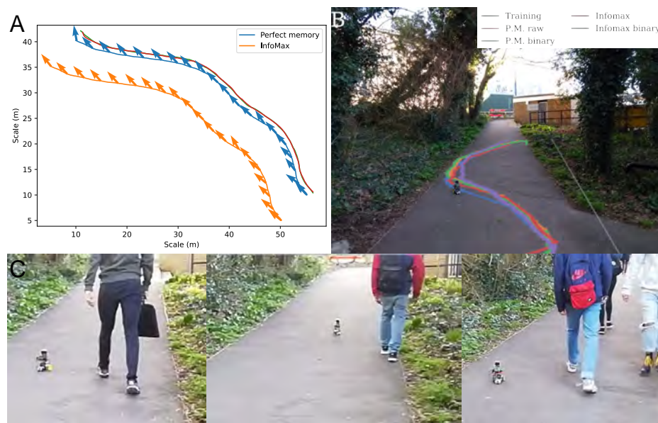
Fig. 6 Route navigation on an autonomous robot. A: Both perfect memory and Infomax provide accurate directions over the ca. 60 m route illustrated in Figure 5B. The red and green lines (the latter is largely obscured by the red) show two passes over the route used for training, the blue shows performance for perfect memory and orange for Infomax. Note that blue and orange routes start at the same starting position as red and green training routes, but have been displaced as they would otherwise obscure each other; the axes are purely for scale. The arrows show the estimated heading direction given at each test point for the two algorithms. B: Closed-loop trials show that route following also works on a real robot platform in a real-world environment. The robot has a panoramic camera and finds its heading by performing periodic scans of the visual scene in silico , then heading in the most familiar directions, after first traversing the blue training route. To assess robustness to contrast changes, we used raw images as well as images automatically converted to binary as sky/not-sky (see legend). C: Performance is not seriously affected by conspicuous changes to the visual scene, such as passing pedestrians.
