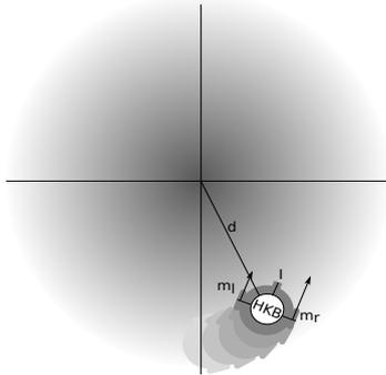
Figure 2: Agent and its environment. The agent has a sensory input, two motors  $m_r$  and  $m_l$  and is controlled by the HKB equation, see Eq. (1). The gradient in the environment is represented by the grey scale, where the darker the color the higher the gradient. The highest gradient is positioned at the coordinates  $x = 0$  and  $y = 0$  in the two-dimensional environment.
