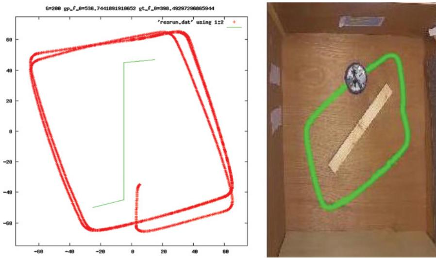
Figure 6: Obstacle avoider trace of fittest controller in a typical run, in simulator (left) and in real arena (right). The real robot trace was produced by processing an overhead video of the robot behaviour with motion tracking algorithms.
