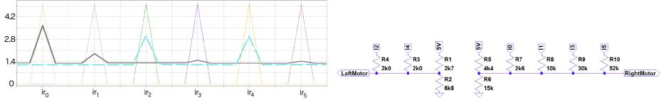
Figure 1: (left) Simulated avoider left motor (dashed) and right motor (thick solid) controller output voltage response to individual IR inputs (thin) ramping up to 5V and down.(right) Minimal reduced implementation of evolved obtacle avoider controller.
