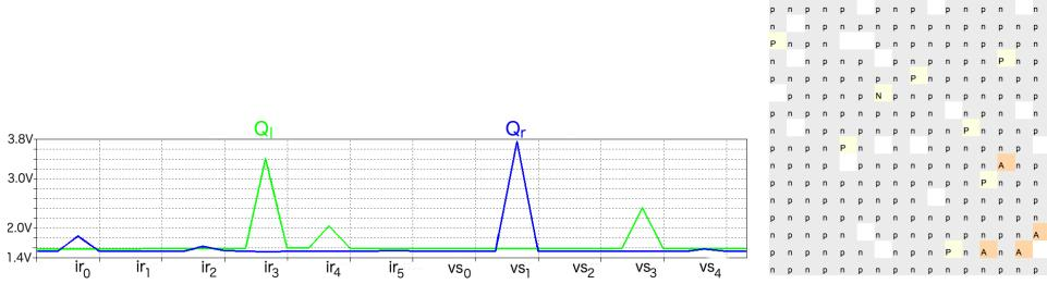
Figure 2: (left) Simulated maze homing controller motor output voltage response to individual IR and visual inputs (ramped as in Fig. 1),  $Q_l$  and  $Q_r$  are left and right motor outputs. (right) Maze homing controller FPTA schematic of cells clamped off (grey), on (yellow) and unclamped (orange).
