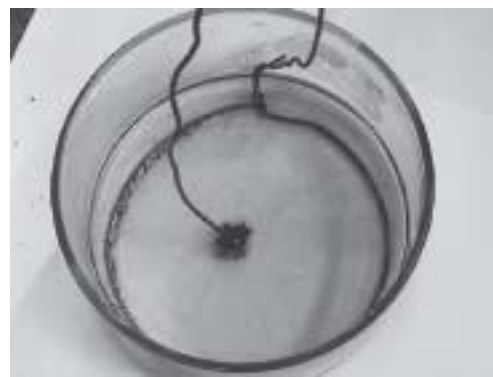
Fig. 5. The experimental setup for growing the thread shown in Fig. 4. A central copper cathode is surrounded by a circular anode. The solution is copper sulfate mixed with sulfuric acid.
