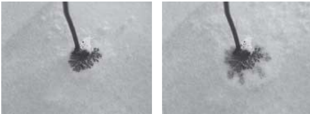
Fig. 4. Photographs of a thread growing on a piece of filter paper. (© Jon Bird) The thread is growing radially from the central copper cathode out to a circular copper anode. See Fig. 5 for an overview of this experimental setup.
