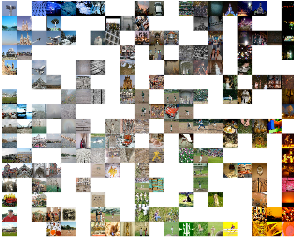
Figure 2: Layout of 320 images into a 2D grid of size 16 by 20 using Self-Organizing Map (SOM). Gaussian neighborhood and inverse learning rate functions are used. For SOM, several images are mapped to the same neuron and some neurons are left with no images assigned. This creates the blank spaces in the visualization. For the neuron with multiple images assigned, we only display one of the images assigned to it.
