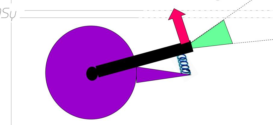
Add a **tentacle**, that can also rotate around the centre. ... with a **photosensor** with an 'angle of acceptance' ... and a **jet** that converts light input into sideways force and a **spring** restraining the tentacle to the nose
