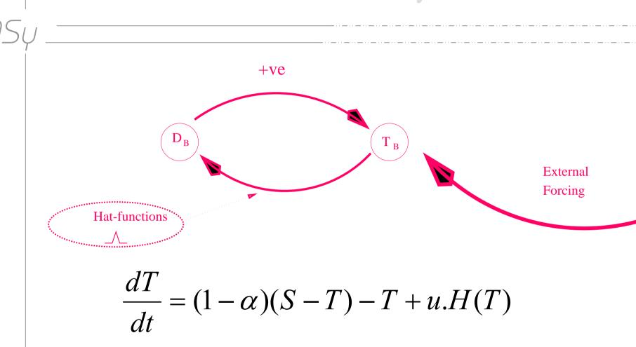
Rate of change of Temp = albedo \* (Suntemp – Temp) – Temp + Feedback-term \* Hat-function(Temp)
