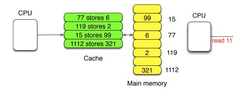
Cache failure on read (highly simplified)
