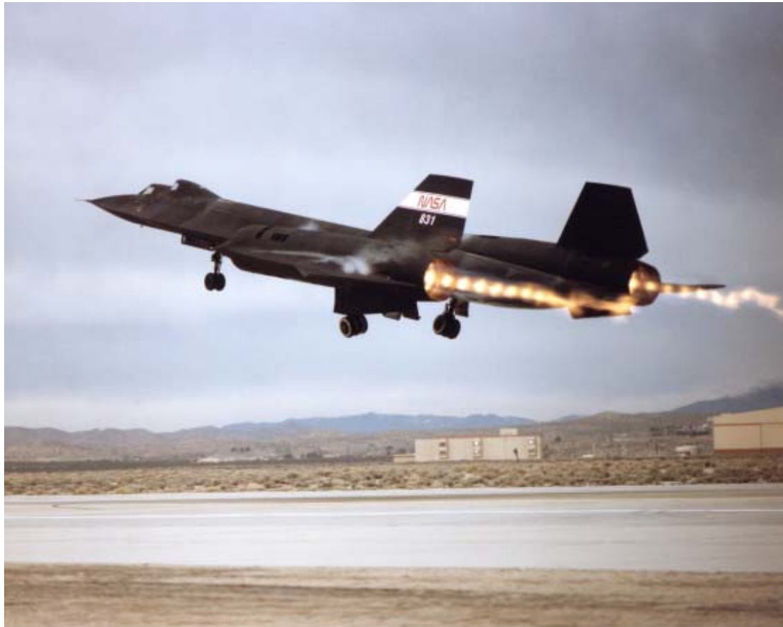
Dryden Flight Research Center EC92-1284 Photographed 1992 SR-71B take-off with "shock diamonds" in the exhaust. NASA photo
