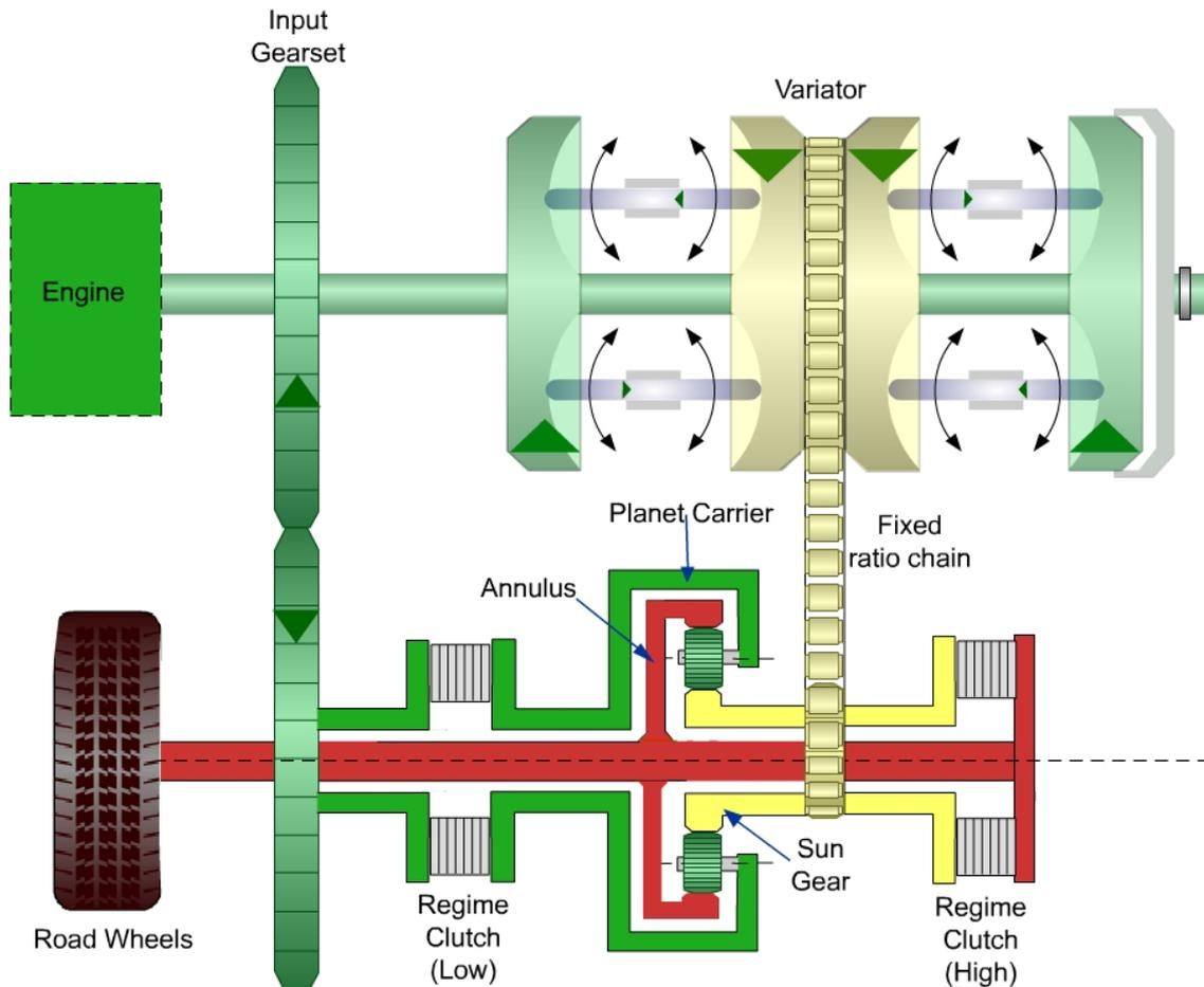
Torotrak use a “split path” layout with an epicyclic gear on the output side. This gives a geared neutral and hence infinite ratio and also a reverse, hence is an IVT.
