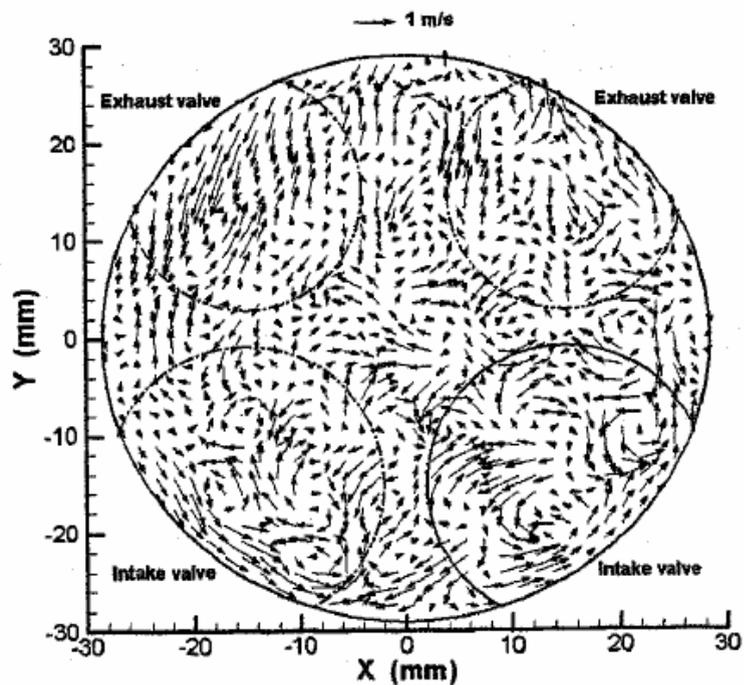
(f) High-frequency fluctuating velocity field
