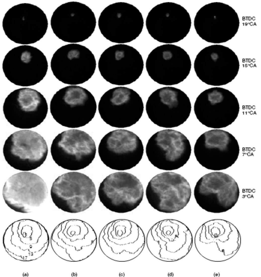
Figure 1. Typical flame propagation patterns in case of (a) without EGR, (b) EGR#1, (c) EGR#2, (d) EGR#3, (e) EGR#4 (number: crank angle after ignition (°CA))
