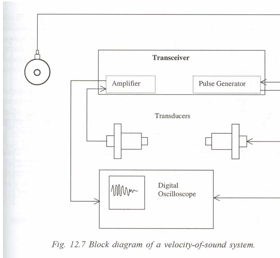
Fig. 12.7 Block diagram of a velocity-of-sound system.
