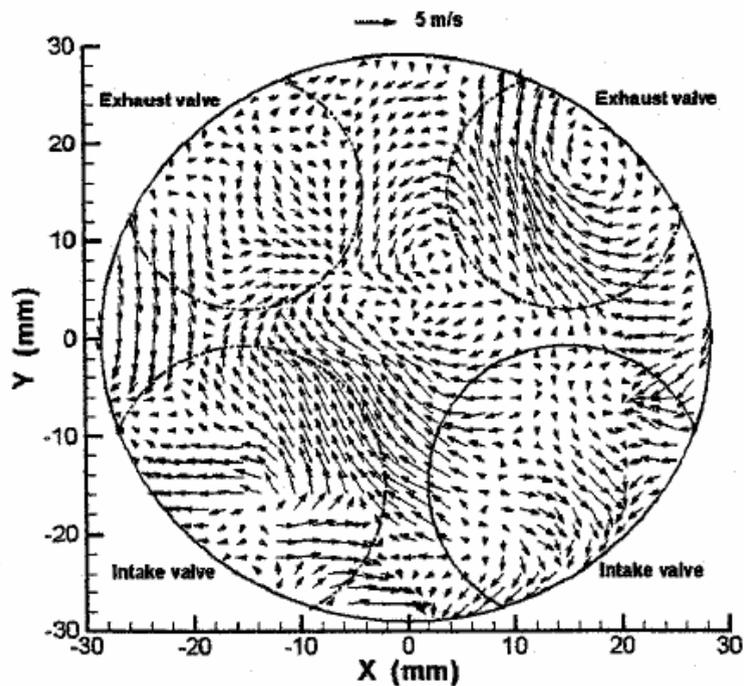
(e) Low-frequency fluctuating velocity field
