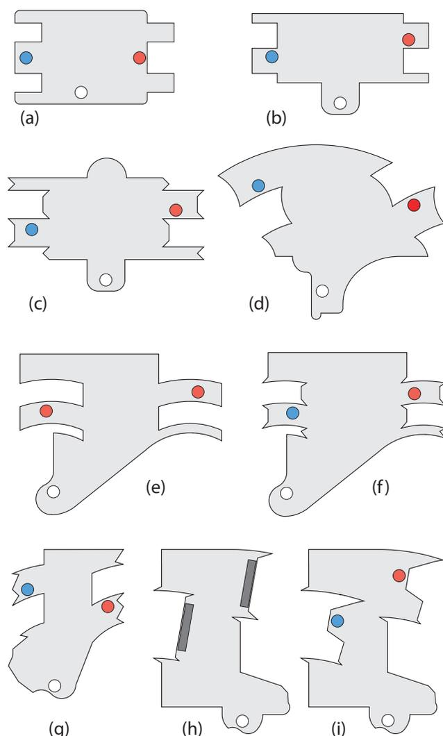
**Figure 6:** A selection of unsuccessful iterations of the design, illustrating the ways in which various issues were solved. The designs are shown in chronological order. See text for details. Magnets are shown in red or blue depending on whether the north or south pole is oriented upwards. The weak bond magnets, whose orientation depends on the polymer type, are shown in white.
