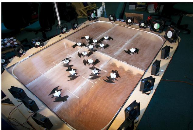
**Figure 2:** The design of the air-hockey style table containing the monomers. Sails on each monomer are blown by a perimeter of small fans. Another fan below the table passes air through small holes to suspend monomers over the table like small hovercraft.
