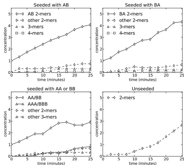
**Figure 9:** Time series data from the same trials as Figure 8, with the reaction products split up by length. Note in particular the drop in concentration of AA and BB dimers towards the end of the trial as they are converted into AAA and BBB via elongation at staggered ends. (Error bars are omitted because they would be overlapping)
