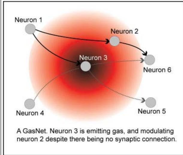
A basic GasNet showing positive (solid) and negative (dashed) “electrical” connections and a diffusing virtual gas creating a “chemical” gradient. [Color figure can be viewed in the online issue, which is available at [wileyonlinelibrary.com](http://wileyonlinelibrary.com).]
