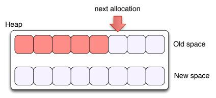
Only the Old space is used in the current round. Allocation is simple: just use next free memory at allocation pointer.
