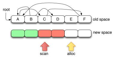
Left of the scan pointer, objects are processed (all pointers have been rewritten). The memory between scan and alloc is copied, but some pointers are still poining to the Old space. Memory from alloc on is free.
