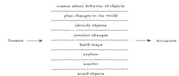
Fig. 2. Decomposition of a mobile robot control system based on task-achieving behaviors.
