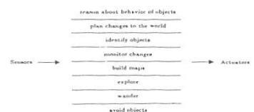
Fig. 2. Decomposition of a mobile robot control system based on task-achieving behaviors.
