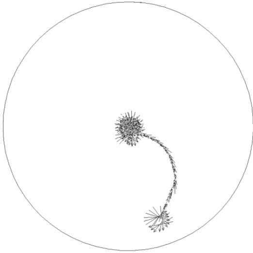
Figure 4: Typical path of a successfully evolved robot, which heads fairly directly for the centre of the room and circles there, using input from 2 photoreceptors. The direction the robot is facing is indicated by arrows for each time step, largely superimposed.
