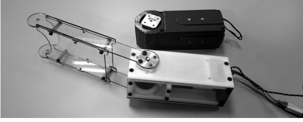
Fig. 3. A photograph of the prototype actuator used in our preliminary work (bottom) with a lever attached to the output and (top) the next generation prototype. The approximate size of the actuator is 50 x 50 x 160mm.
