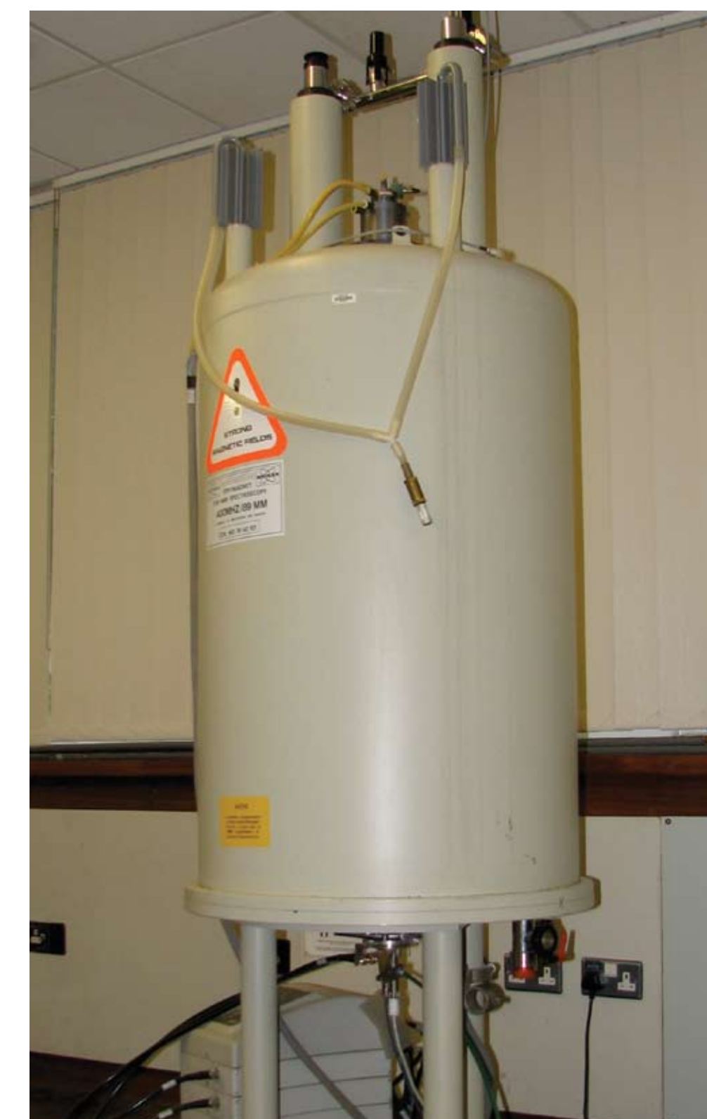
Bruker Avance DMX 400 MHz 9.4 T / 89 mm Spectrospin Magnet 4mm ^{31}\text{P} - ^{15}\text{N}\{^1\text{H}\} MAS Probe ^1\text{H} gHR-MAS Probe 10 mm ^{31}\text{P} - ^{109}\text{Ag}\{^1\text{H}\} solution probe
