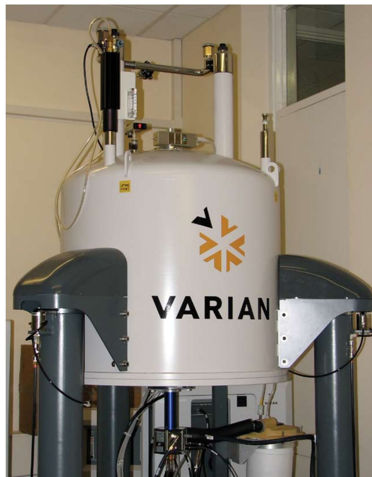
Varian VNMRS 400 MHz 9.4 T / 54 mm Premium Shield Magnet ^1\text{H} - ^{19}\text{F}/^{31}\text{P} - ^{15}\text{N} AutoX DB Probe
