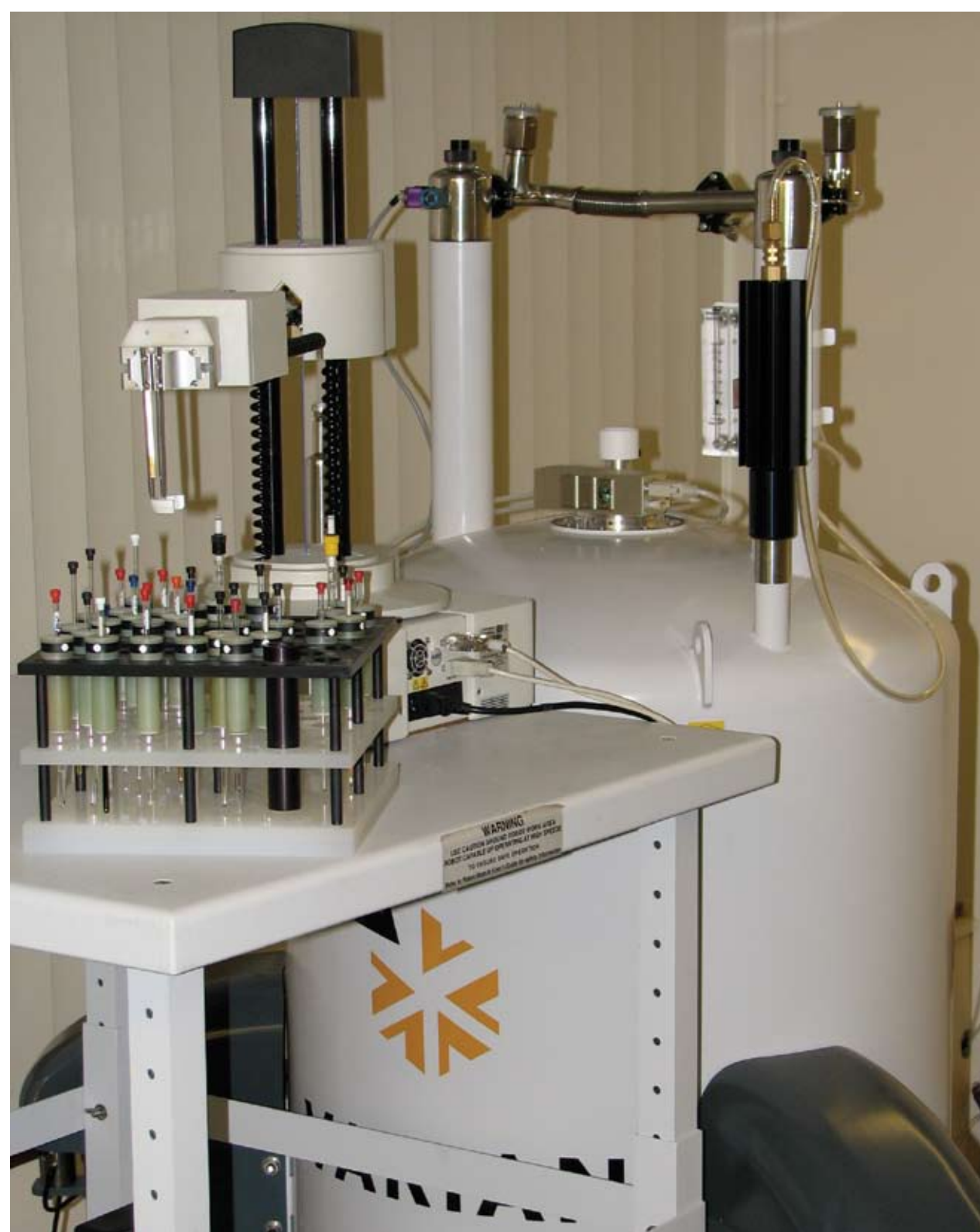
Varian VNMRS 500 MHz 11.75 T / 54 mm Premium Shield Magnet ^1\text{H}\{^{31}\text{P} - ^{15}\text{N}\} AutoX ID Probe SMS-50 Autosampler
