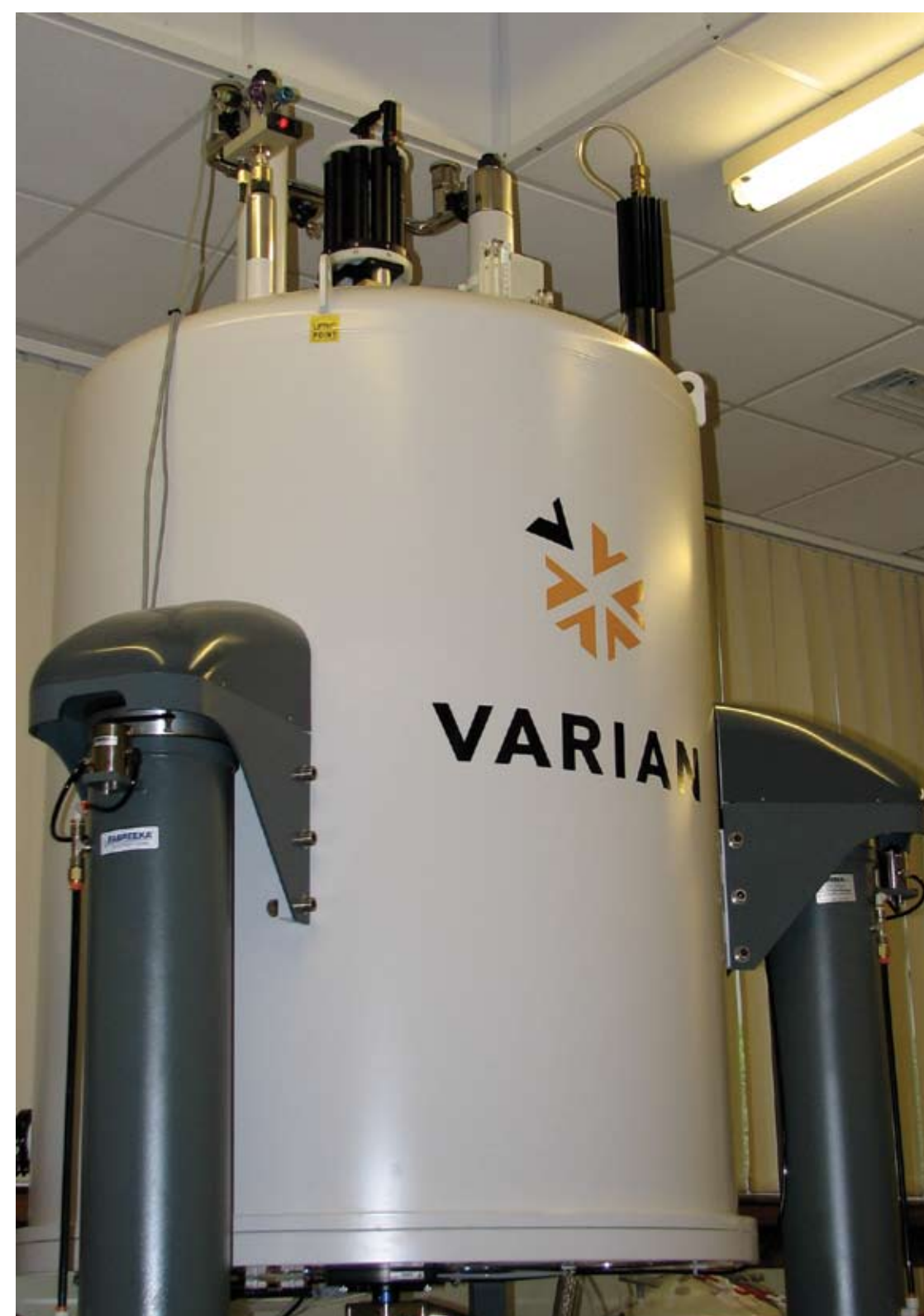
Varian VNMRS 600 MHz 14.1 T / 54 mm Premium Shield Magnet ^1\text{H} - ^{19}\text{F}/^{31}\text{P} - ^{15}\text{N} AutoX DB Probe ^1\text{H}\{^{31}\text{P}/^{13}\text{C}/^{15}\text{N}/^2\text{H}\} AutoPenta Probe 9 Sample Carousel
