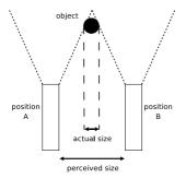
Figure 3: The 'inverse shadow' effect. Assuming the device is moving from left to right, the user will start perceiving the object at position A and stop perceiving it at position B. The object's apparent size is bigger than its actual size.
