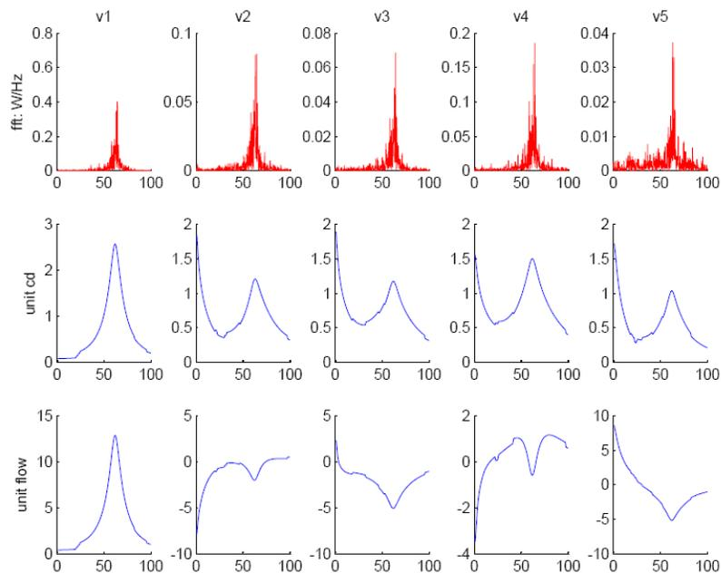
**Figure 2.** The top row shows the power spectrum for each variable (node), assuming a sampling rate of 500 Hz. The middle and bottom rows show the by-variable causal density and causal flow, following a spectral G-causality analysis. Note that peaks in the causal density spectra coincide with peaks in the power spectra. Note also that y-axes have different scales.
