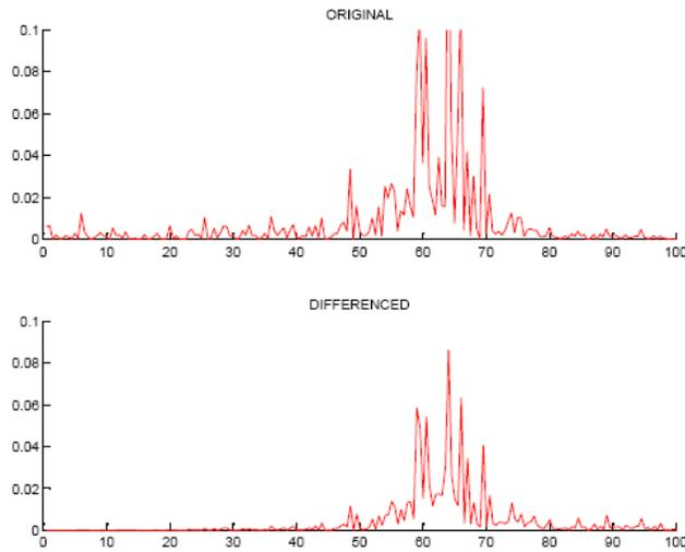
**Figure 7.** Fourier spectra for original (top) and differenced (bottom) time-series. In this case, the power spectrum is mostly preserved, but it is not identical. In other examples, the post-differencing power spectrum can appear grossly distorted, especially if prior to differencing the bulk of power was in the lower frequency range.
