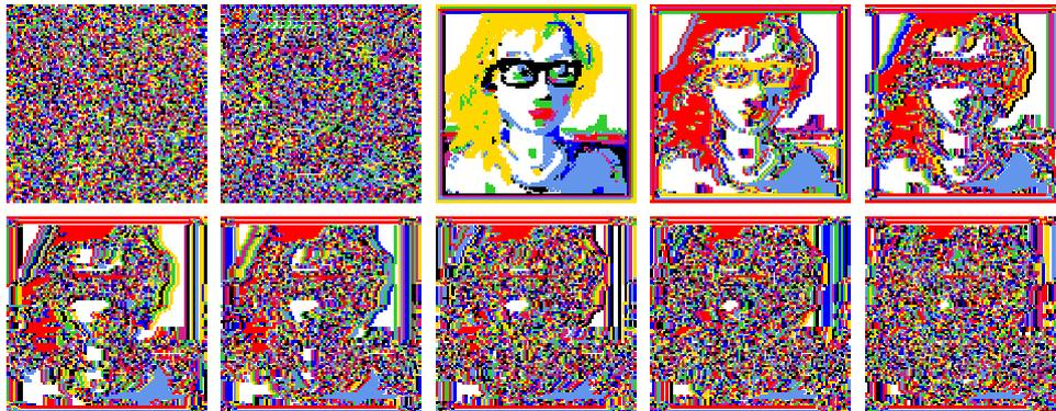
Fig. 15. To decrypt, starting from the encrypted state in Fig. 14 ( $n=7744$ ,  $88\times 88$ ), the CA with the same  $v=8$  chain-rule was run forward to recover the original image. This figure shows time-steps -2 to +7 to illustrate how the image was scrambled both before and after time step 0.
