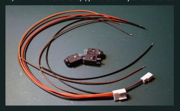
The Z cable needs to be about 6 inches longer than the X/Y if you want to poke the cables out of the bottom of the case.
