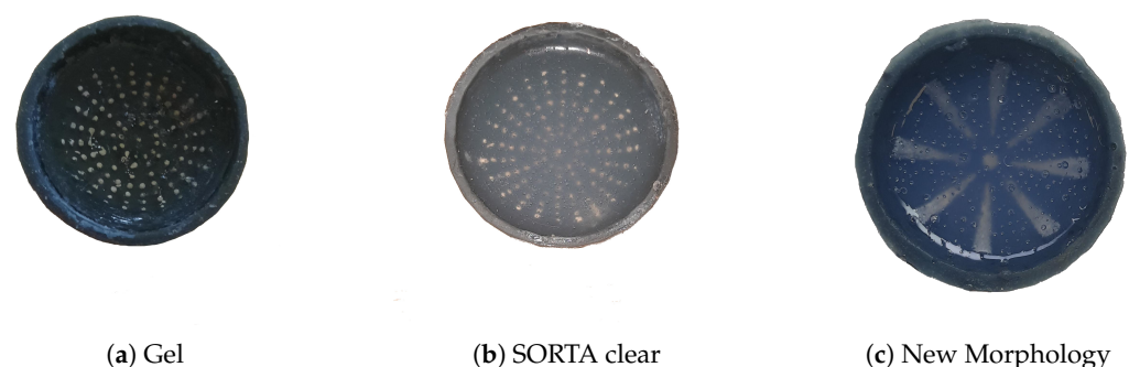
Figure 1. The different soft bodies for the skin of the TacTip. (a) The RTV27905 Gel in the original TacTip; the cloudier adaptations in (b,c) use the cheaper clear silicone, with (c) being the lower resolution design.
