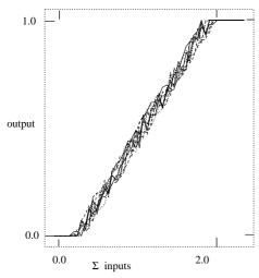
Figure 2: Noisy neuron transfer function.
