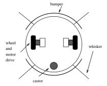
Figure 1: Plan view of simple six-sensor robot.
