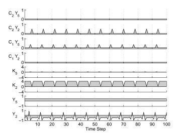
Figure 3: For nodes 2 (the right-back motor node) and 5, involved in the 'spiking' subnetwork, the figure shows data over a run of 100 time-steps for node output  $Y \in [-1,1]$ , node transfer parameter  $K \in [-4,4]$ , positive and negative gas concentrations  $C_1, C_2 \in [0,1]$  at the node site. Area between the output and time axis is shaded for clarity.
