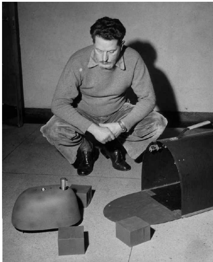
Figure 4: Grey Walter watches one of his tortoises push aside some wooden blocks on its way back to its recharging hutch. Circa 1952.
