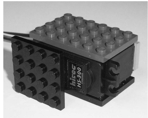
Figure 1: The controller has Lego parts glued to it allowing it to be attached to other parts.
